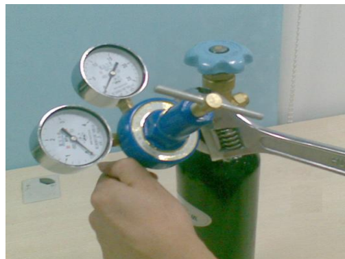
(2) The intake pipe pressure reducing valve
