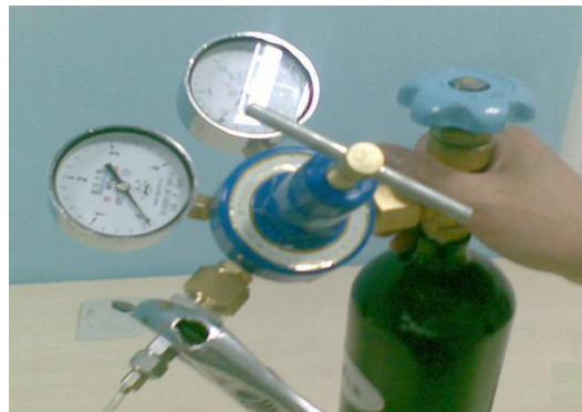
(3) The intake pipe connecting instrument air inlet
